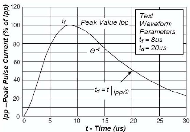
**Fig1. Pulse Waveform**
