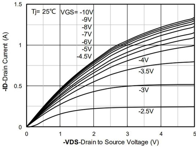
Figure 1. Output Characteristics
