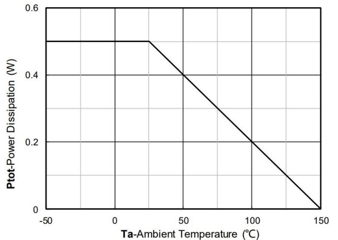
Figure 12. Power dissipation
