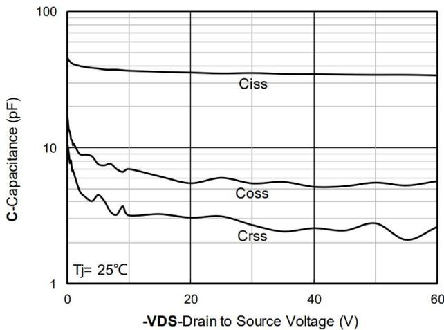
Figure 3. Capacitance Characteristics
