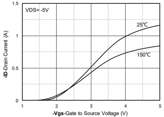
Figure 2. Transfer Characteristics
