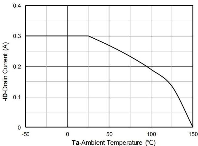
Figure 11. Current dissipation
