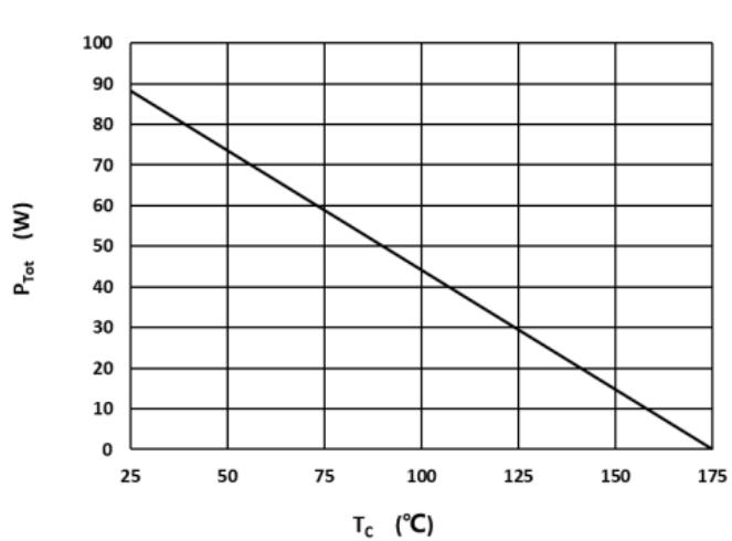
Figure 6. Power dissipation as function of case temperature
