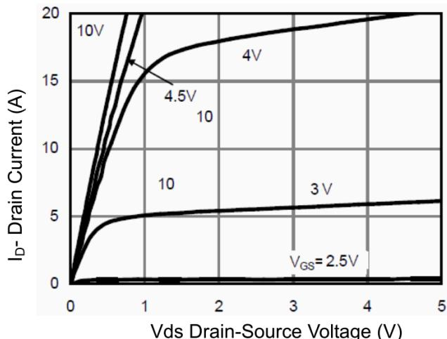
Figure 1 Output Characteristics
