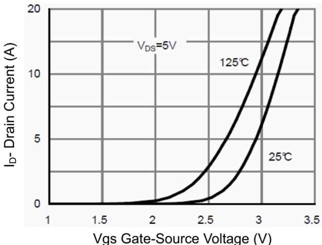
Figure 2 Transfer Characteristics
