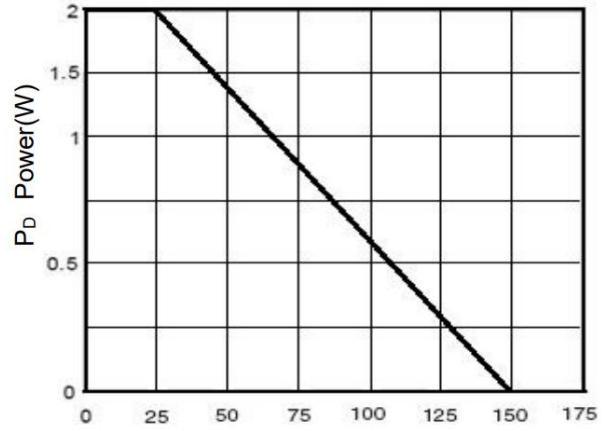
T J -Junction Temperature(°C) Figure 8 Power Dissipation
