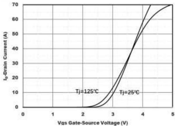
Figure2. Transfer Characteristics
