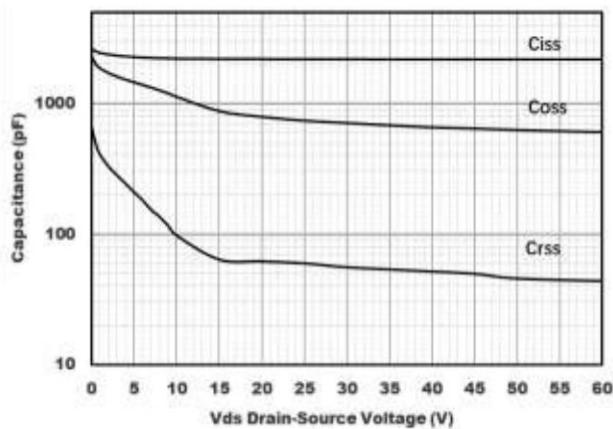
Figure3. Capacitance Characteristics
