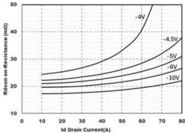
Figure5. : On-Resistance vs. Gate to Source Voltage
