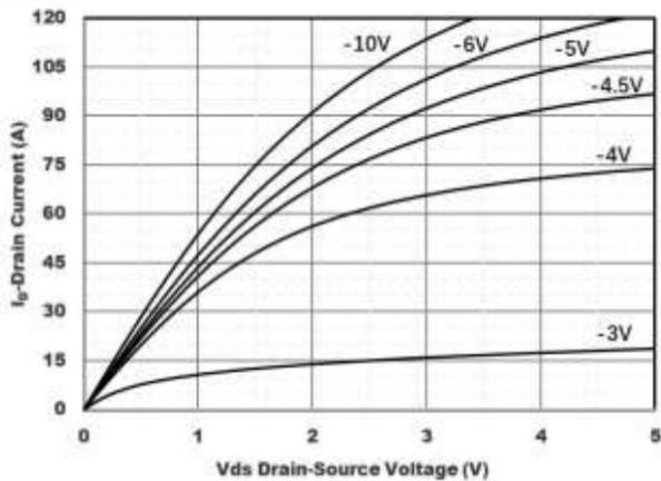
Figure1. Output Characteristics
