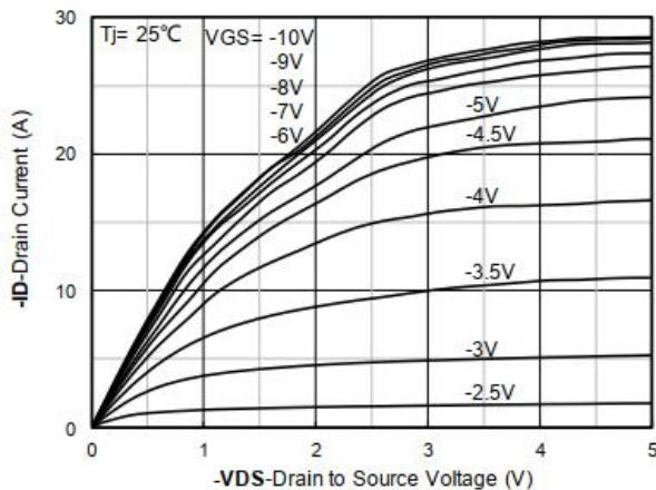
Figure 1. Output Characteristics
