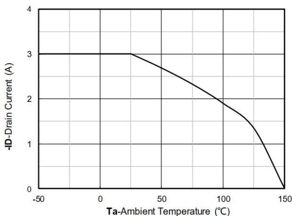
Figure 11. Current dissipation
