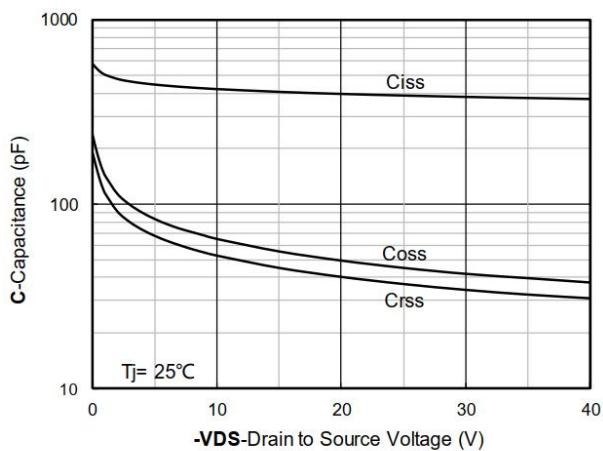
Figure 3. Capacitance Characteristics
