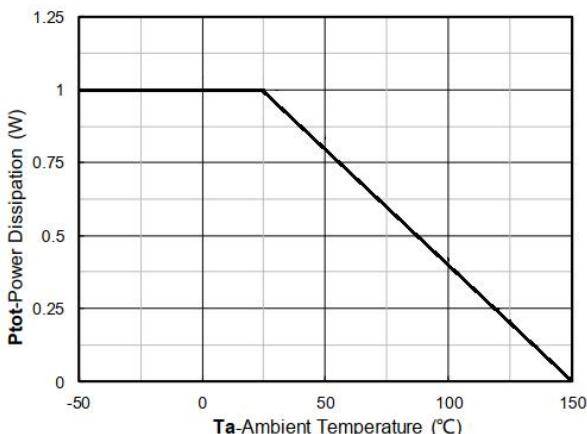
Figure 12. Power dissipation
