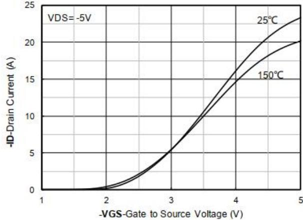
Figure 2. Transfer Characteristics
