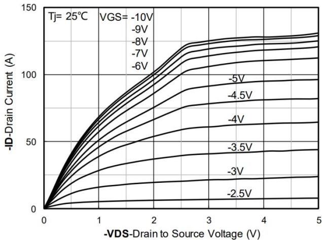
Figure 1. Output Characteristics
