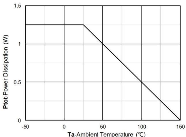
Figure 12. Power dissipation
