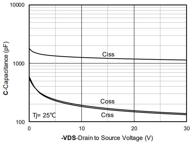
Figure 3. Capacitance Characteristics
