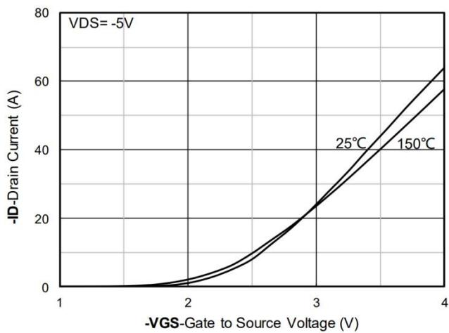
Figure 2. Transfer Characteristics
