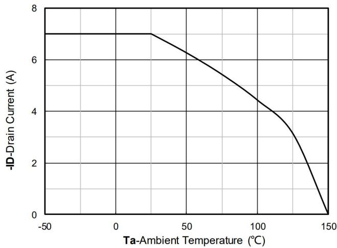
Figure 11. Current dissipation
