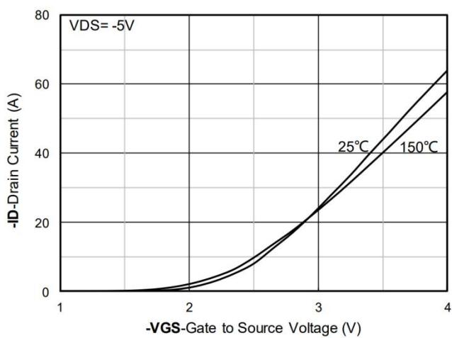
Figure 2. Transfer Characteristics
