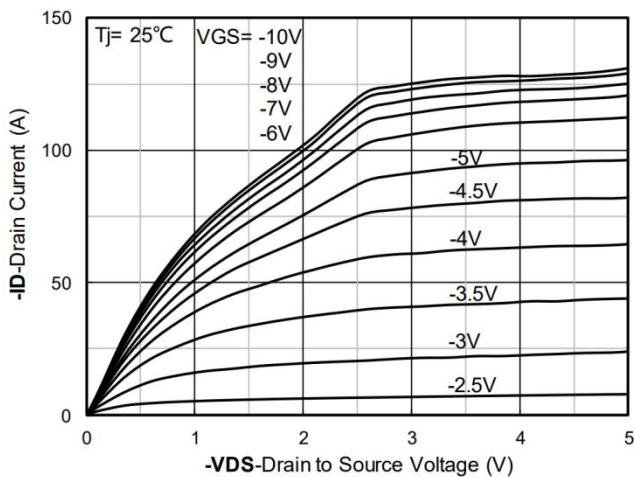
Figure 1. Output Characteristics
