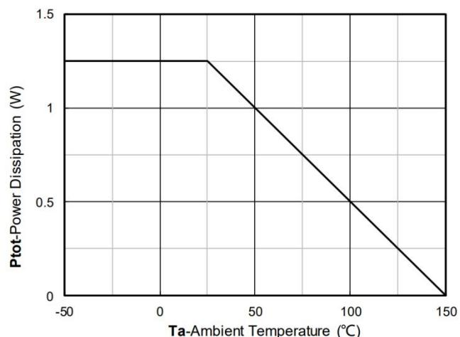
Figure 12. Power dissipation
