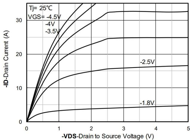
Figure 1. Output Characteristics
