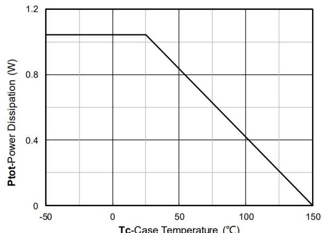
Figure 12. Power dissipation
