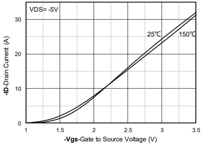
Figure 2. Transfer Characteristics
