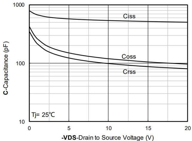
Figure 3. Capacitance Characteristics
