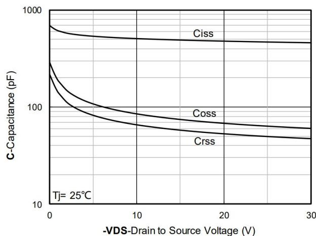
Figure 3. Capacitance Characteristics
