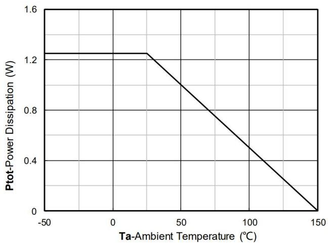
Figure 12. Power dissipation
