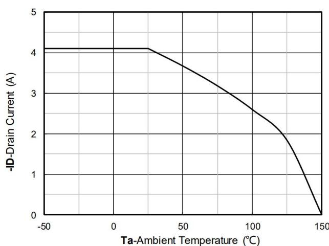
Figure 11. Current dissipation
