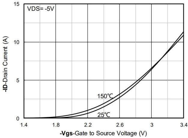
Figure 2. Transfer Characteristics
