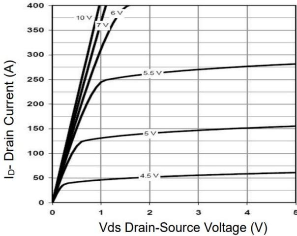
**Figure 1 Output Characteristics**
