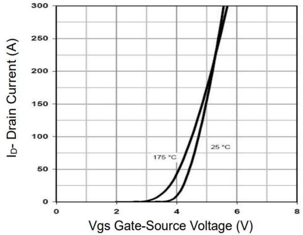
**Figure 2 Transfer Characteristics**
