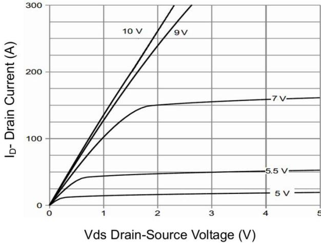
**Figure 1 Output Characteristics**
