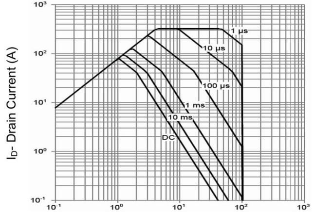
V<sub>ds</sub> Drain-Source Voltage (V)
