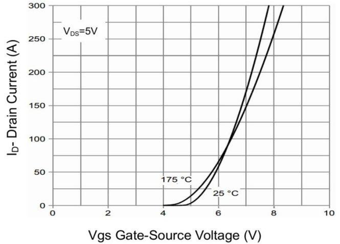
**Figure 2 Transfer Characteristics**
