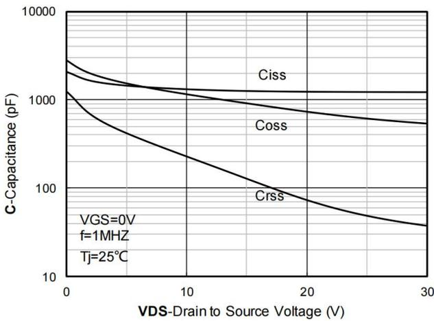
Figure 3. Capacitance Characteristics
