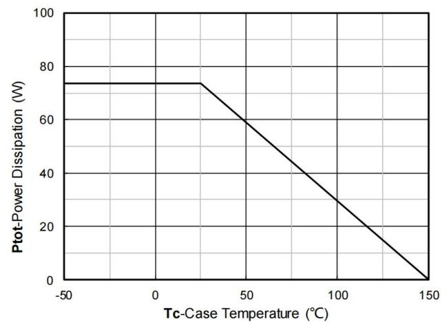
Figure 12. Power dissipation
