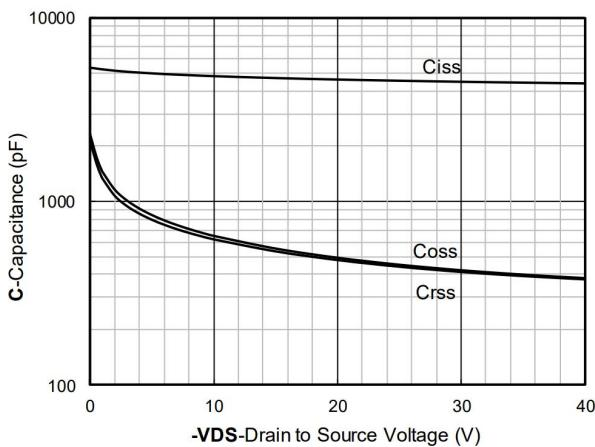
Figure 3. Capacitance Characteristics
