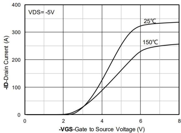
Figure 2. Transfer Characteristics
