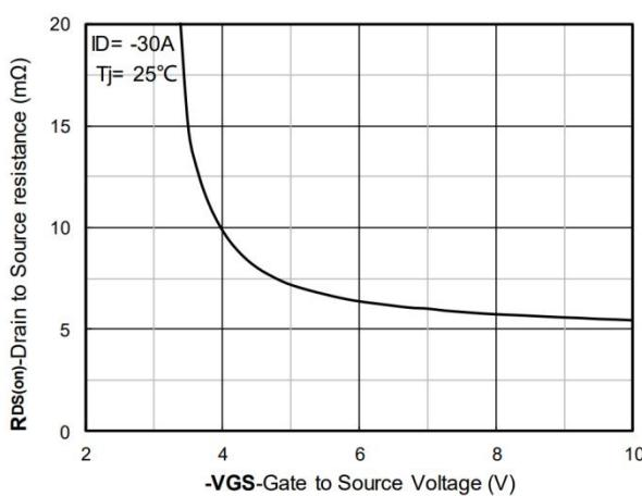
Figure 5. On-Resistance vs Gate to Source Voltage
