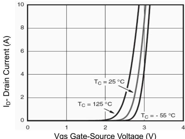
Figure 2 Transfer Characteristics
