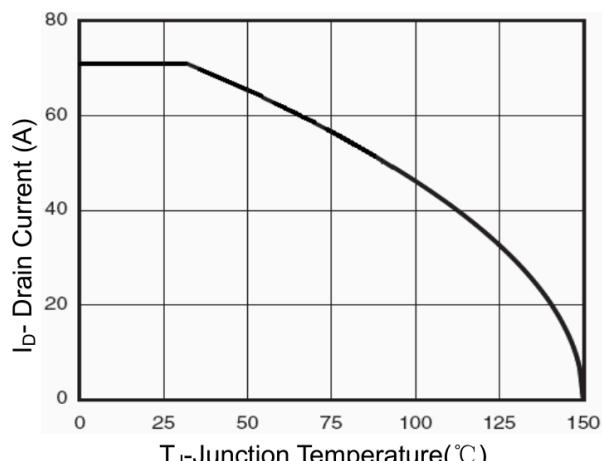
Figure 10 ID Current Derating vs Junction Temperature
