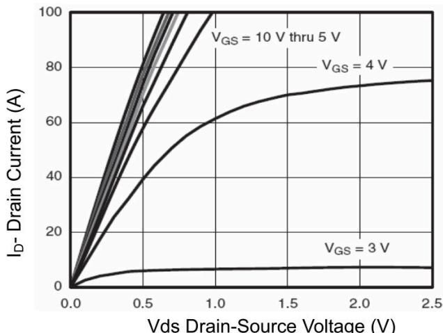
Figure 1 Output Characteristics
